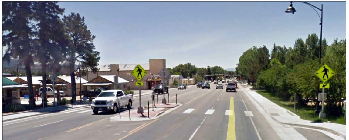
Mid-block crossing and Rectangular Rapid Flashing Beacons (RRFBs) on State Highway 24 (CO-24), in Buena Vista, Colorado.
