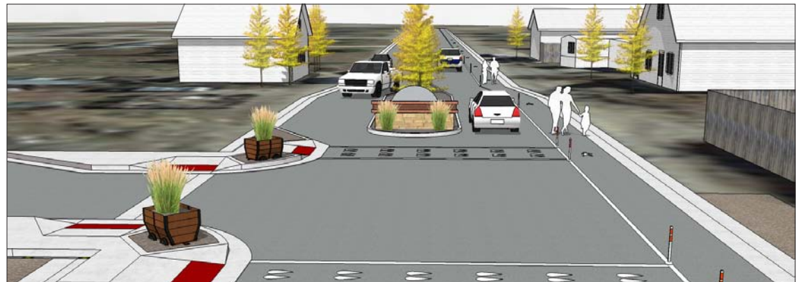
Concept for permanent curb extensions at the intersection of 6th Street & Front Street.
